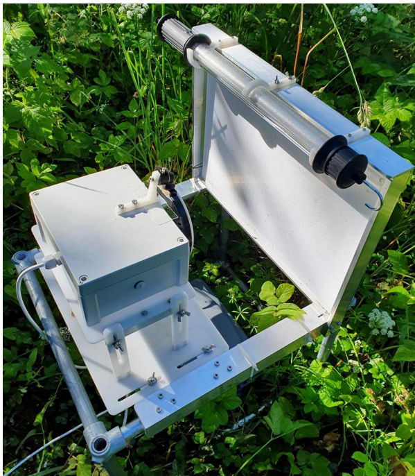
Figure 1. Camera trap with UV light to attract and monitor nocturnal insects.
